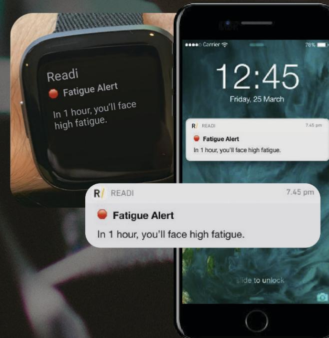
**Fatigue Alerts, for when it matters most:** Operators receive vibrating reminders on their wrist and phone when they are approaching a period of critical fatigue.
